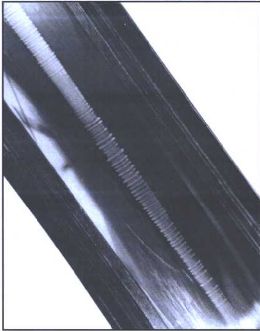
Figure 2. Fluting of the Bearing Race Caused by Current Discharged through the Bearing Lubricant
